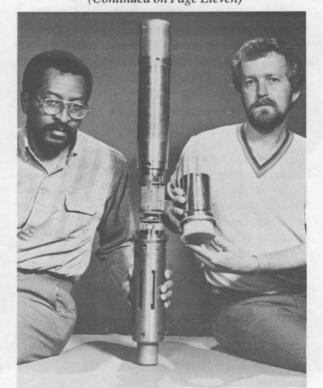
FRED HEARD (left, now 9234) and Tom Bauman (now 9127) teamed for development of the geothermal high-temperature, high-pressure acoustic borehole televiewer. Fred holds acoustic sensor assembly — motor, rotating transformer, magnetometer, and transducer. Tom displays a magnetometer pressure housing section.
